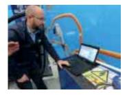
The only way the vehicle can be made safe is by using the VAG diagnostics tools, by logging into VW Audi Germany via ODIS. There is no other way of safely "de-energising" the vehicle without damaging the car. Once these instructions have been followed, the maintenance
